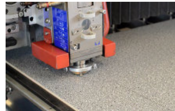
Customized shaping of the platform with laser cutting
